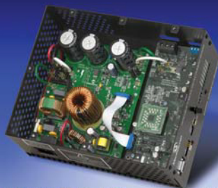
dsPICDEM™ MCHV Development Board (Part # DM330023)
